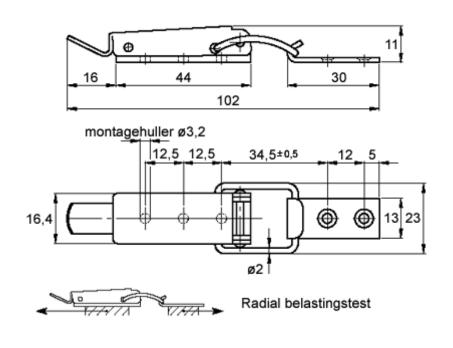
$\begin{array}{l} \text{Max load (N)} &= 550 \\ \text{Ultimate strength (N)} &= 1200 \end{array}$
